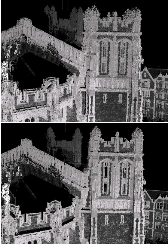
Figure 9: Shepard Hall. Close up view of pairwise registration. (Top) With automated registration before ICP optimization. Range scans do not align perfectly. (Bottom) After ICP optimization. Result has been significantly improved.
