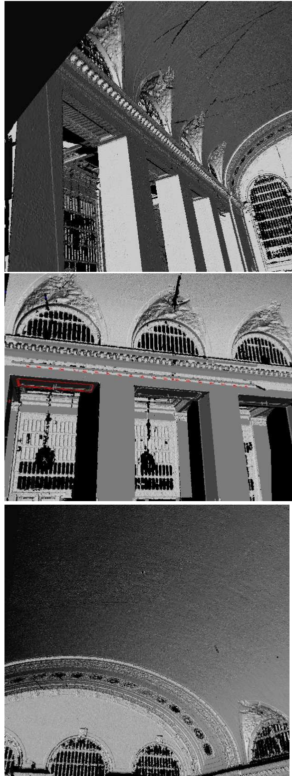
Figure 5: (Top) 3D model constructed via an implementation of the ball pivoting algorithm. Note that large planar areas around the columns are modeled as dense meshes. (Middle) Hybrid model: planar areas are modeled as large polygons (gray color for clarity), while non-planar areas are modeled via mesh. This representation is closer to a 3D CAD model. (Bottom) Part of the model that is modeled as mesh.
