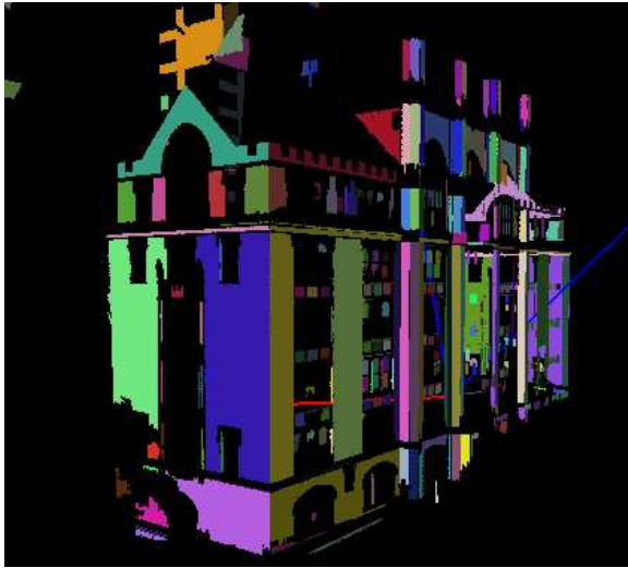
Figure 4: View of the final planar 3D model after all planar segments from ten registered segmented scans are merged. Again, different planes are represented with different colors for clarity.
