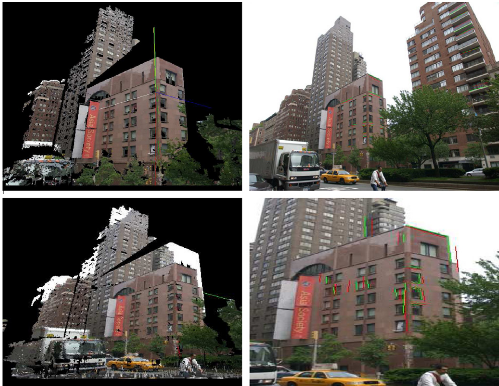
Fig. 9. Asian Society building, NYC. (Top row:) Texture-mapped image on 3D model (left) and 2D image with matched 2D features projected on 3D features (right). Correct transformation. This is the best option provided to the user. Note that lines from nearby buildings have been used for its computation. (Bottom row:) Texture-mapped image on 3D model (left) and part of 2D image with matched 2D features projected on 3D features (right). Incorrect transformation. This is one of the wrong options generated. In that example the rotation is correct, but the translation is not. The error is evident since images of nearby buildings are projected on the 3D model of the Asian Society building.
