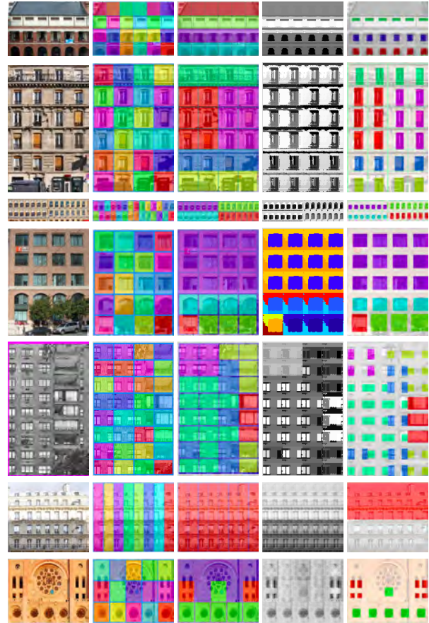
Figure 6. From left to right: follow the order of Fig. 4. First five rows show success cases (robustness to occlusions and different architectural styles). Last two rows are failure cases due to the photometric variation and inability to model via a Kronecker product model.
