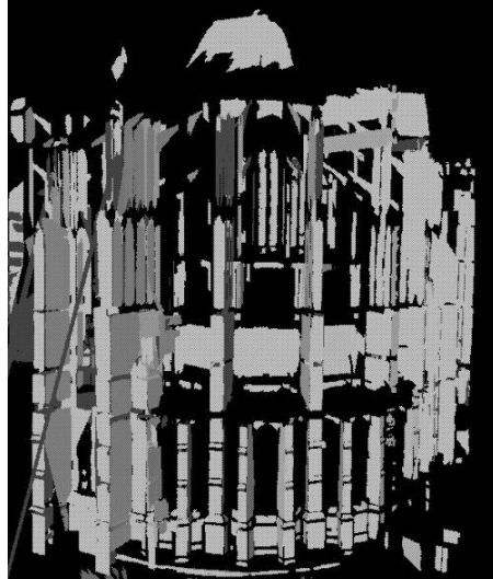
Figure 4: Segmented regions from point cloud.
