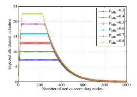
Fig. 8. Idle channel utilization with  $N_T = 30$  and  $N_S = 100$
