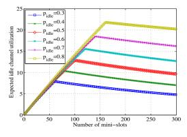
Fig. 7. Idle channel utilization with  $N_T = 30$  and  $\lambda_s = 3$
