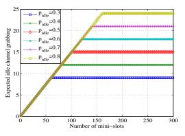
Fig. 5. Idle channel grabbing characteristics, with  $N_T = 30$  and  $\lambda_s = 3$ .
