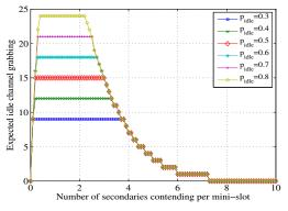
Fig. 6. Idle channel grabbing characteristics with  $N_T = 30$  and  $N_S = 100$
