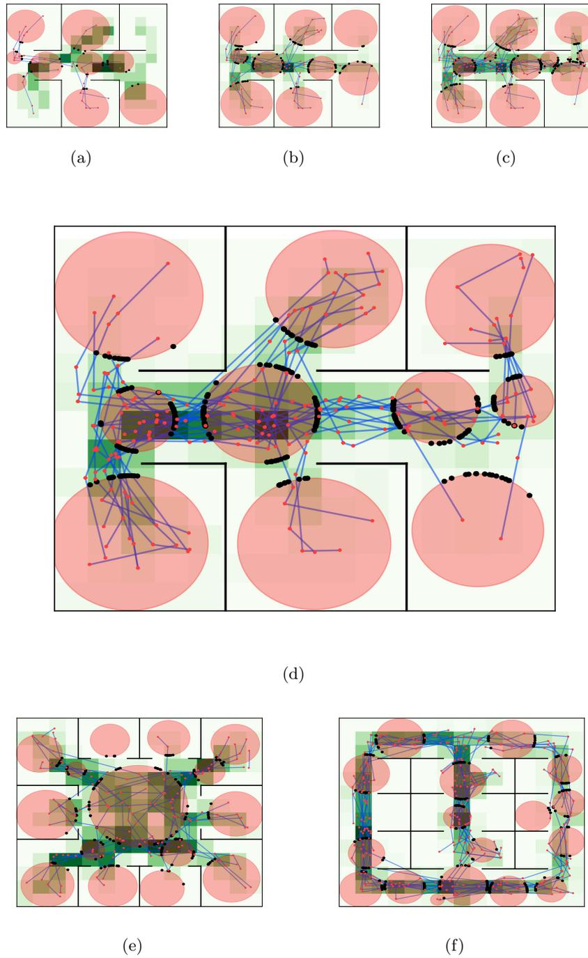
**Fig. 4.** Spatial models in SemaFORR, overlaid on the corresponding true map, which the robot does not have. Conveyors are shown as grid cells (darker is more salient), and regions as circles with dotted exits. Trails are line segments with dots at the trail markers. The spatial model for world A as it evolves after (a) 10 (b) 20 and (c) 30 targets. After 40 targets, SemaFORR's learned spatial models of (d) world A, (e) world B, and (f) world C.
