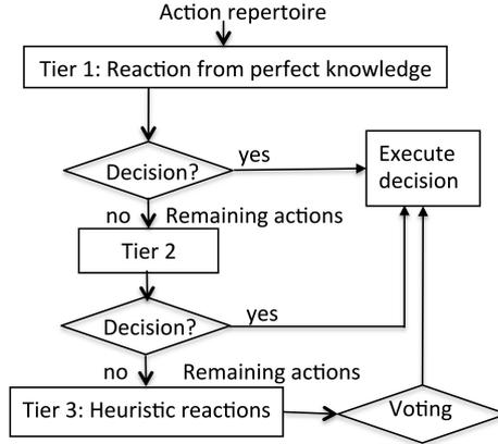
**Fig. 2.** A schematic for SemaFORR’s control structure with sample input.
