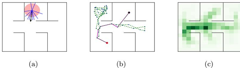
**Fig. 1.** (a) The robot’s position produces values for its wall register, which provides its local view. The arrow represents the robot’s heading; the subtended circle is the detected region. (b) A (dotted) path begun in the lower left room and the (solid) trail derived from it, with dots at the trail markers. (c) A conveyor grid; darker cells are more often crossed by trails.
