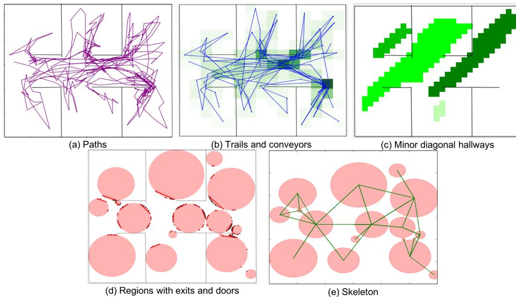
■ **Figure 1** Affordances in a learned spatial model after visiting 40 randomly-assigned locations in a simple world (a) paths taken by the robot (b) trails refined from paths and overlaid on conveyors shaded by their count (c) minor diagonal hallways (d) regions with exits (points on the perimeter) and doors (secants) (e) the skeleton. Horizontal and vertical lines are not part of the model; they represent physical walls.
