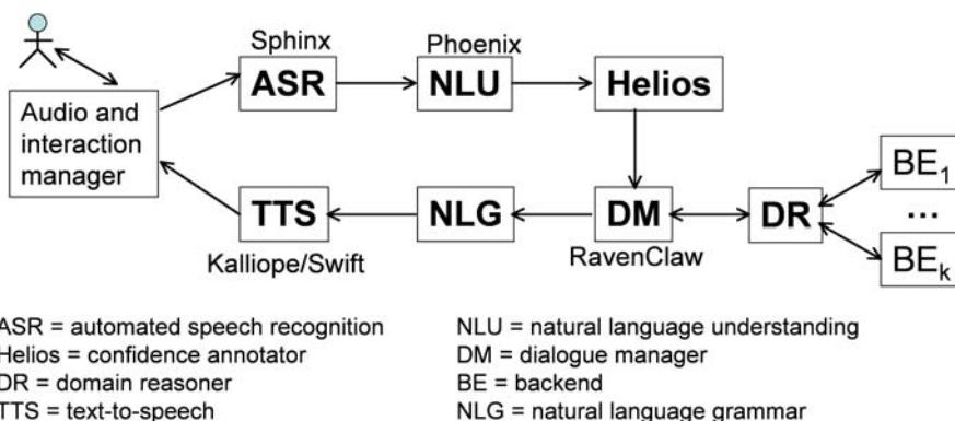
Figure 3: The Olympus/RavenClaw dialog system. Errors in automated speech recognition impact every module in the system.
