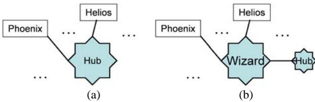
Figure 5: Rewiring (a) the Olympus/RavenClaw star topology to (b) incorporate the wizard.
