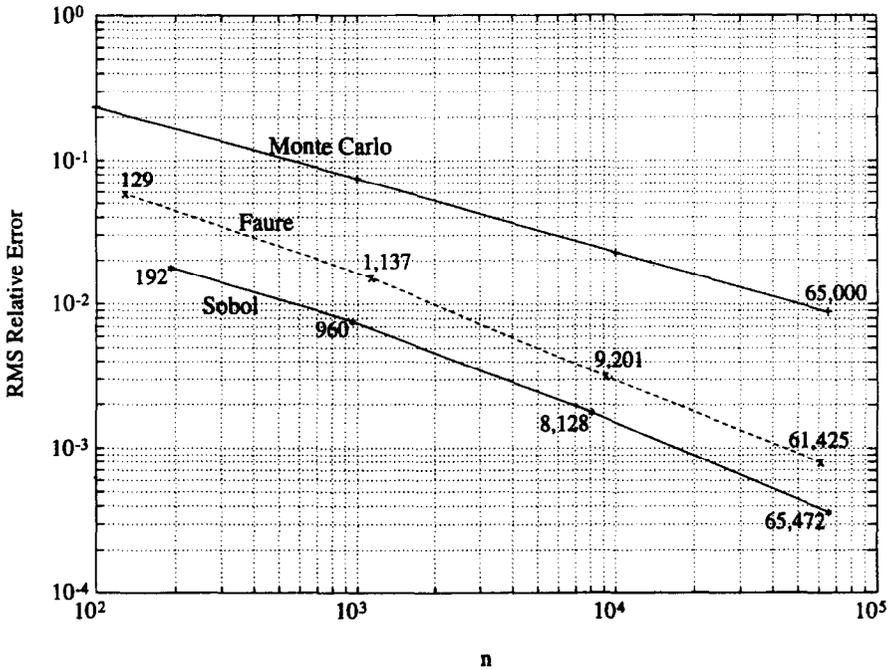
Fig. 1. RMS relative error vs. number of points.
