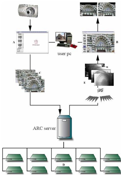
**Figure 10. Schematic overview of the client-server setup. Images (C) are uploaded from the upload tool (A) on the user side to the server. There they are processed on a PC cluster (D). The results (E) can be downloaded via ftp and visualized on the user PC with the modelviewer tool (B).**
