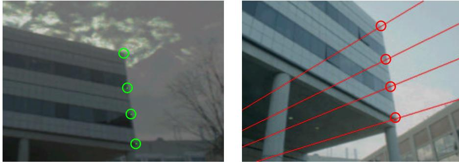
**Figure 26: AmesCourt Epipolar Geometry**
