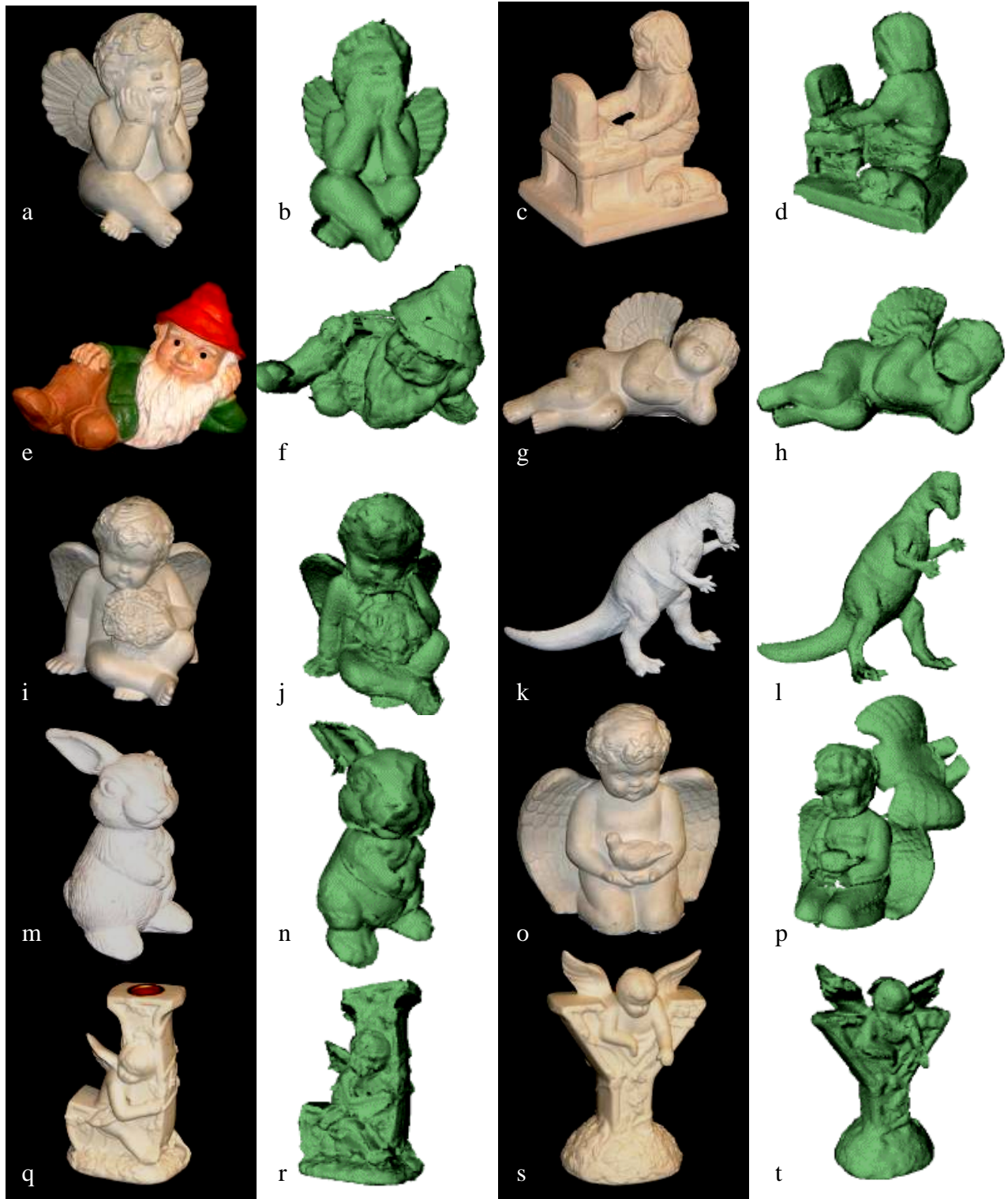
Fig. 9. Photographs of the ten test objects (first and third columns) and the resulting 3D models (second and fourth columns). a-b) angel1; c-d) coder; e-f) dwarf; g-h) angel2; i-j) angel4; k-l) dino; m-n) rabbit; o-p) angel3; q-r) letter_j; s-t) letter_y.
