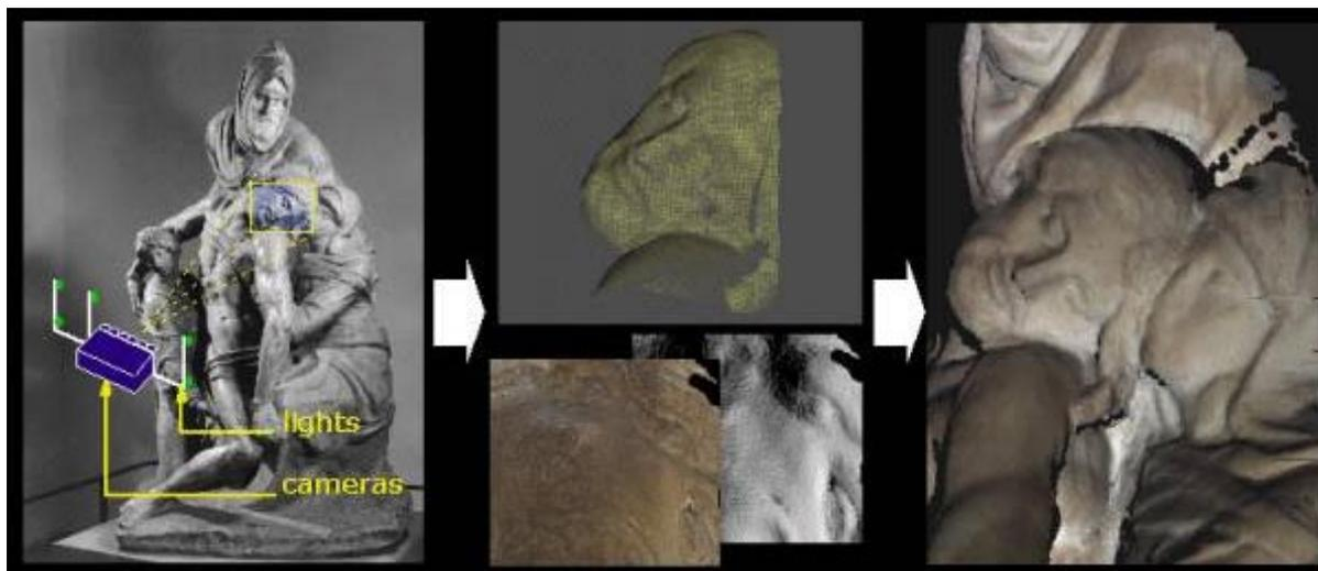
Fig. 2. 3D capture methodology: (a) Multiple digital photos are taken. (b) Surface shape, color and details are computed for each scan. (c) Scans are aligned and merged into a single model.
