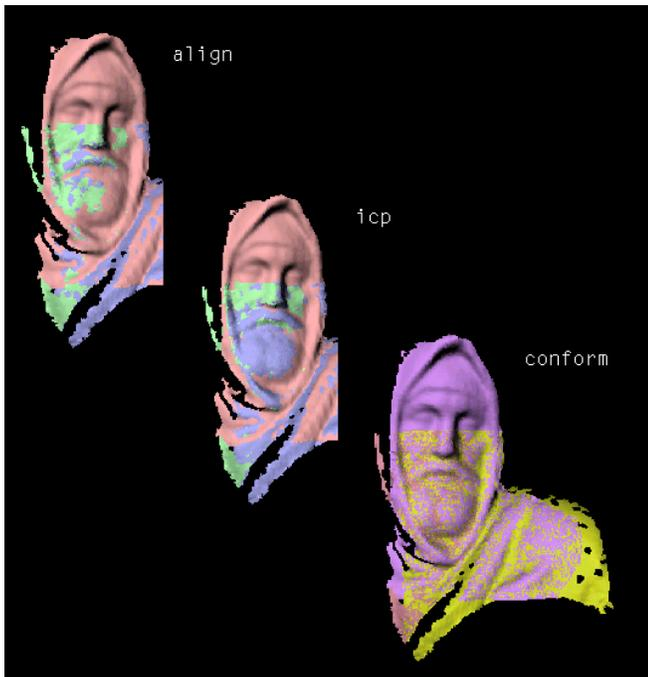
Fig. 5. Subsequent steps of the registration of three test scans. Each scan is shown with a different color. In the “conform” step the scans have been slightly deformed (and so shown with a changed color) to compensate for residual registration and measurement error.
