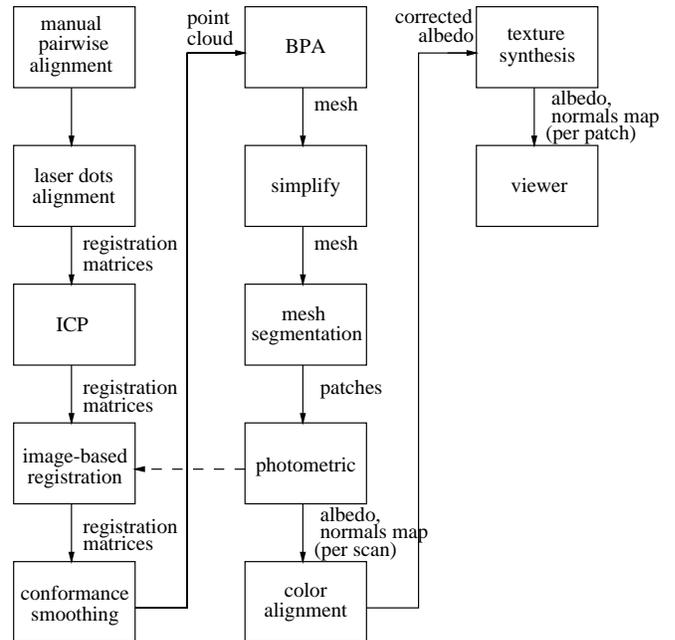
Fig. 4. The reconstruction pipeline.
