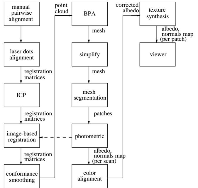
Fig. 4. The reconstruction pipeline.
