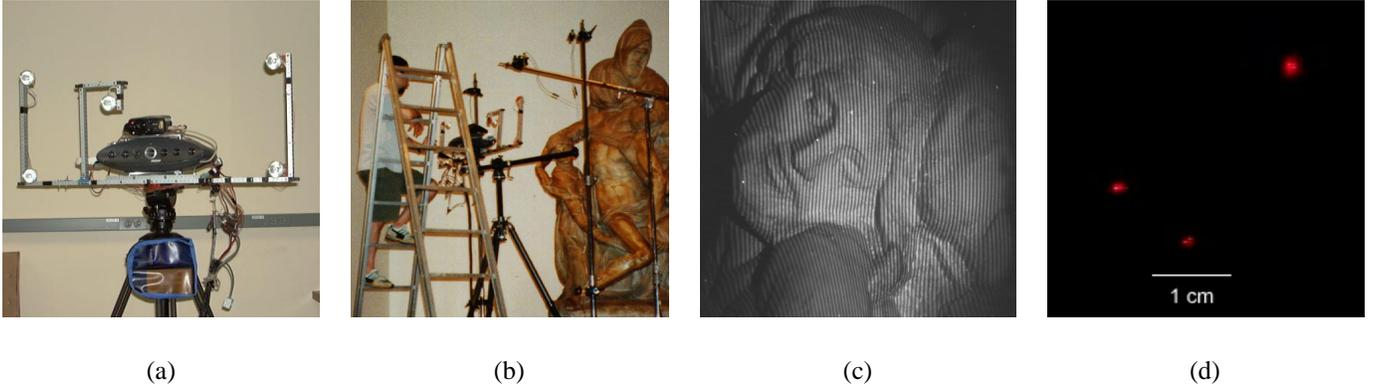
Fig. 3. (a) The scanner used in the project. The five-light photometric system was added to a Virtuoso ShapeCamera. (b) The scanner in use in the museum. The stands visible in the picture are used to hold the laser projectors. (c) Detail of one of the six stripe images simultaneously taken by the scanner. (d) Detail of the laser dots projected on the statue, as captured by the color camera mounted on the scanner.
