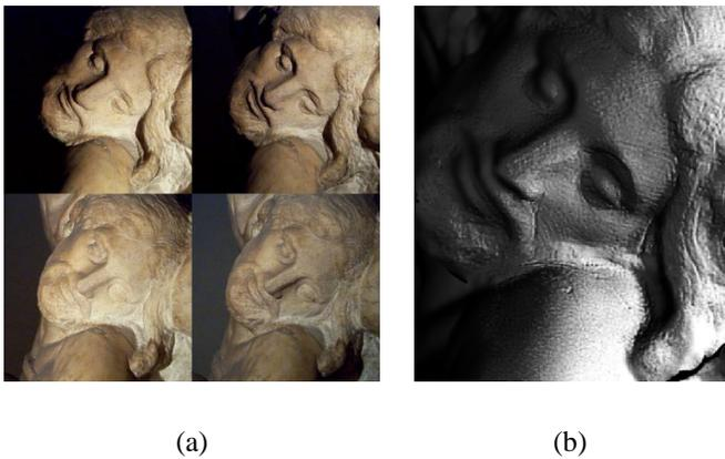
Fig. 6. (a) Color images taken with four of the five light sources. (b) Synthetic picture computed using the surface normals obtained with the photometric system.
