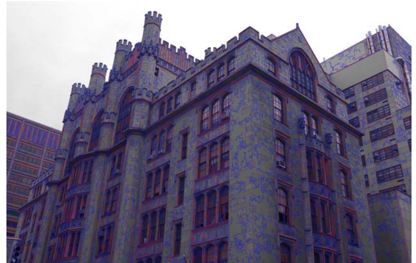
After edge detection (red lines are the lines extracted from blue edges)
