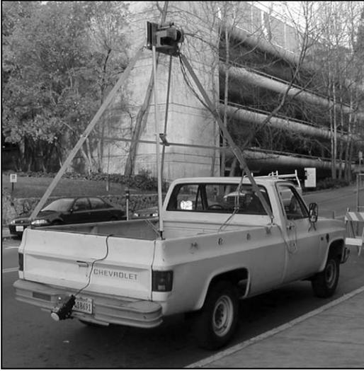
Figure 2. Truck with acquisition equipment.
