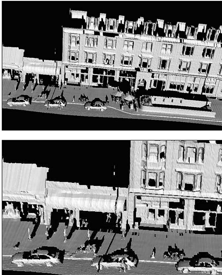
*Figure 21.* Surface mesh by triangulating the point cloud.
