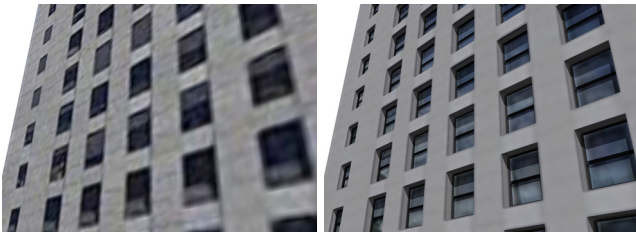
Figure 2: The method can be applied to enhance state-of-the-art oblique aerial imagery. Left: close-up view of original texture (note the blur due to the low resolution). Right: our reconstruction.
