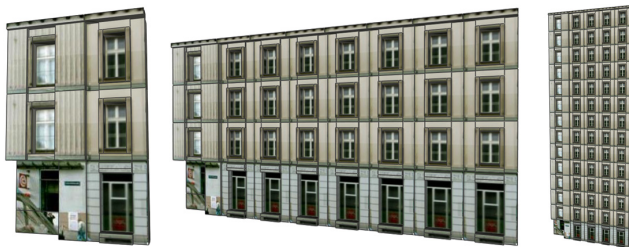
Figure 14: The extracted rule set is size-independent and can be applied to copy-paste the design (or part of) onto other 3D models.
