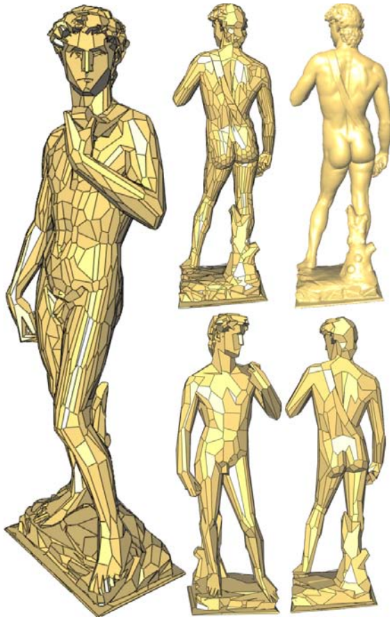
Figure 17: David (700K triangles): at two different resolutions for the L^{2.1} metric (resp. 5 min, and 10 min), front and back views. Edges inside each region are removed to improve clarity.
