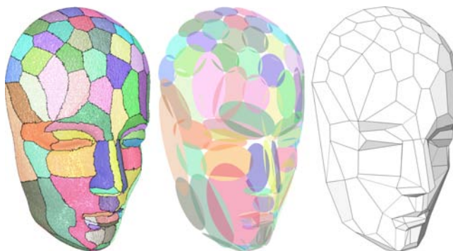
Figure 1: Variational Shape Approximation : Through repeated error-driven partitioning (left), we find a set of geometric proxies (represented as ellipses, center) providing a concise geometric description of an input surface (62K triangles) by efficiently capturing the anisotropy of the initial model; notice the presence of disks on near-spherical regions, and stretched ellipses on near-parabolic regions. These proxies are then used to construct an approximating polygonal mesh (right). No user interaction, parameterization, or differential estimates have been used; total processing time: 3s.
