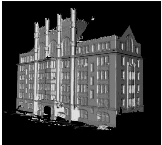
Figure 2: [TOP ROW] (a) & (b) North and south views of the mesh model of the Thomas Hunter Building in New York City. The model was generated with the method of [5]. [MIDDLE ROW] (c) & (d) North and south views of the same model with mesh planar areas  $MPA_s$  identified as blue. [BOTTOM ROW] (e) & (f) 3D model after simplification.
