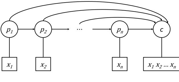
Figure 5. Generalized HMM for jointly classifying a sequence of object parts and object class. Part labels depend only upon part features and joint features with the previously predicted part. Class labels depend on the classification of all parts and their features.
