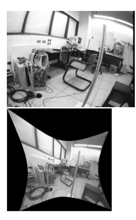
Distorted (up) and undistorted image (down). The computed parameters are:
