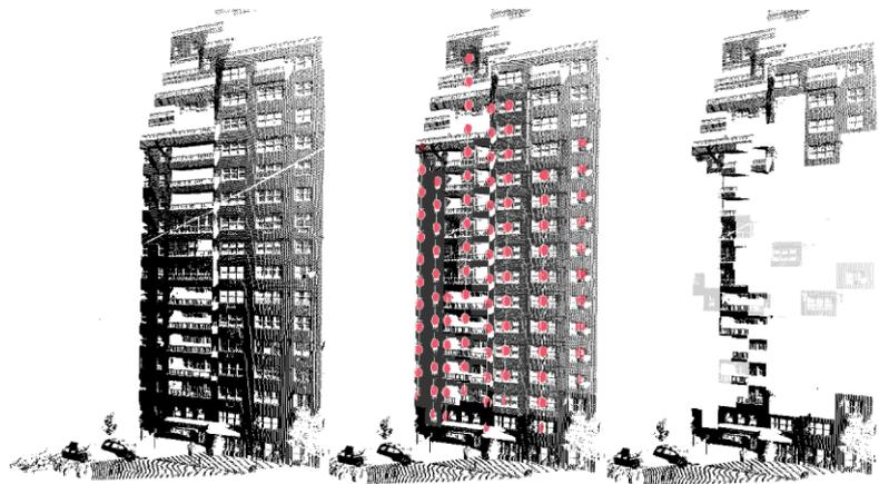
**Fig. 22** Two views were synthesized from a single scan by applying a known transformation  $T$ . Our method then estimates a transformation  $T_*^{-1}$ , using the methods of Sect. 6
