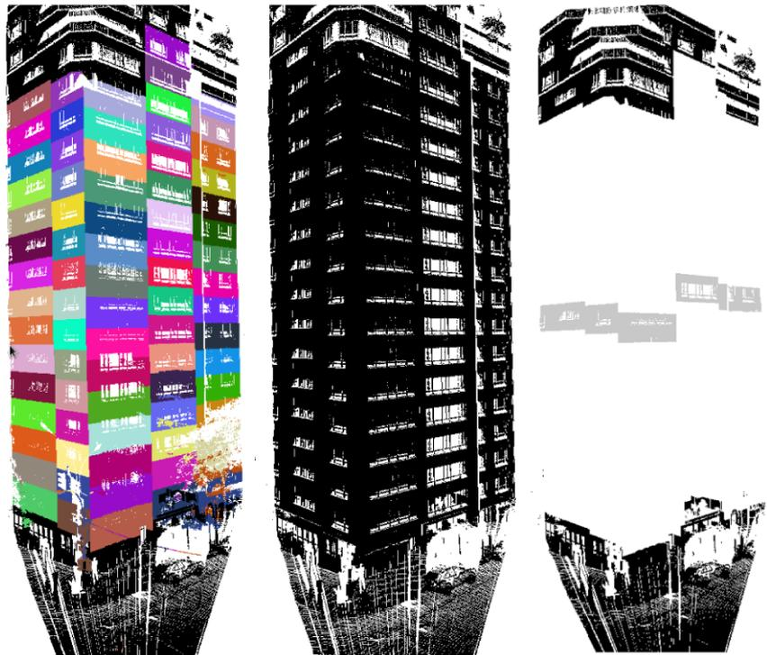
**Fig. 15** The *left* image is a segmented scan. The *middle* image is a compressed version of the scan to the *left*. The *right* image shows the amount of reduction. The *grey points* are the representative regions. The compression ratio is 55 %, with 300628 points removed out of 546964 total points (Color figure online)
