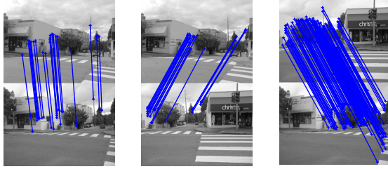
Figure 7: Another example where localization is based on the triangulation and all three motions can be estimated based on fundamental matrix. Left: Identified correspondences between the query view (top) and the first reference view (bottom). Center: Identified correspondences between the query view (top) and the second reference view (bottom). Right: Identified correspondences between the second reference view (top) and the first reference view (bottom).
