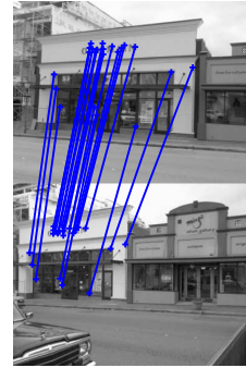
Figure 9: Only one reference view (bottom) can be found for the query image (top), because the query view is "extrapolated".
