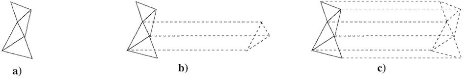
**FIG. 12.** Sweeping triangular mesh elements. (a) Triangular mesh surface, (b) one triangular element swept towards sensing direction, (c) all triangular elements swept.
