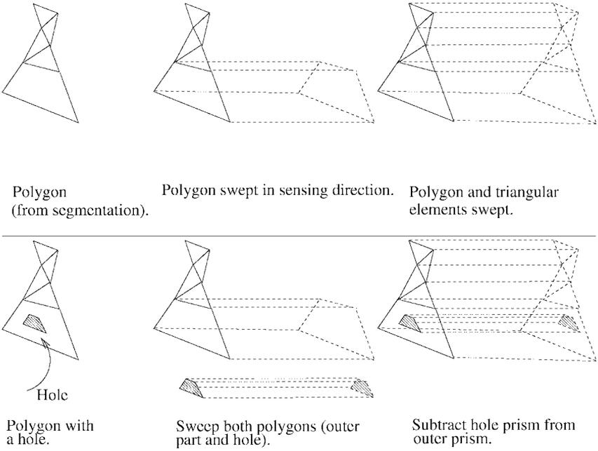
**FIG. 13.** Extension of solid modeler. Top row: (left) Polygonal face (without holes) and triangular mesh elements. (middle) One polygonal element swept toward the sensing direction. (right) All elements swept. The union of all prisms is the resulted partial solid volume. Bottom row: same concept. Now, though, the polygonal face has holes.
