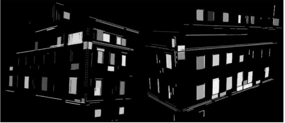
**FIG. 17.** (a,b) Clusters of 3-D lines (color encodes different directions) and extracted 3-D rectangles (rectangles are rendered as solids of different color for clarity). Two different views of the building.
