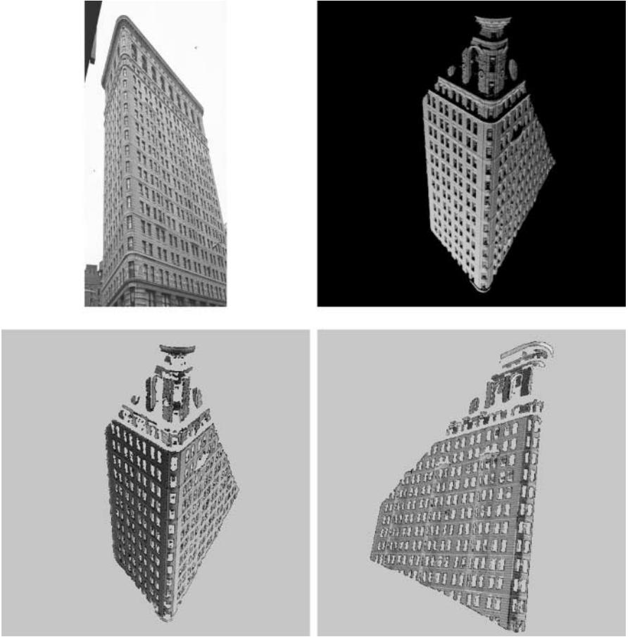
**FIG. 9.** Flat-Iron Building. Top row: Two-dimensional photograph and dense range scan (first view). Bottom row: Segmented range scans (first and second view). Each segmented surface is displayed with a different color. The points which failed the initial *Point Classification* step are displayed in red.
