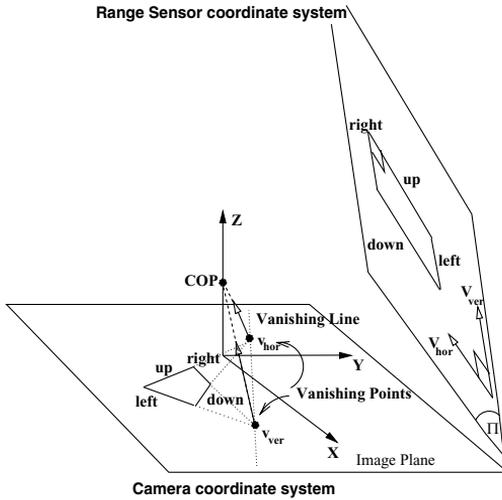
**FIG. 16.** 3-D rectangle formed by lines parallel to the scene directions  $V_{ver}$  and  $V_{hor}$  and its corresponding 2-D quadrangle formed by 2-D lines which meet at the image vanishing points  $v_{ver}$  and  $v_{hor}$ .
