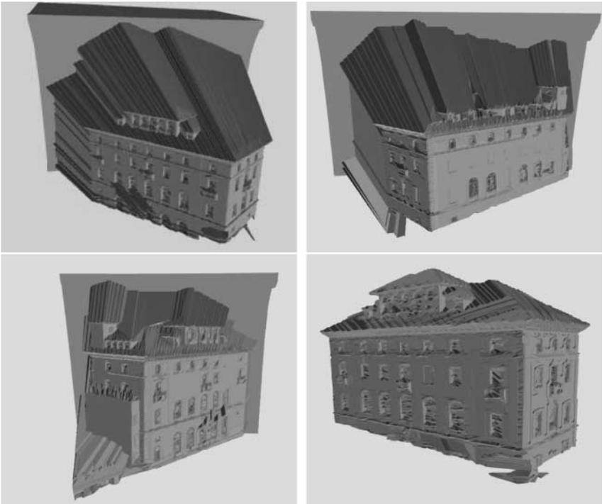
**FIG. 14.** Modeling Casa Italiana. Three volumetric sweeps of the segmented range scans. The volumetric set intersection of the three sweeps leads to the final composite solid model (bottom right image).
