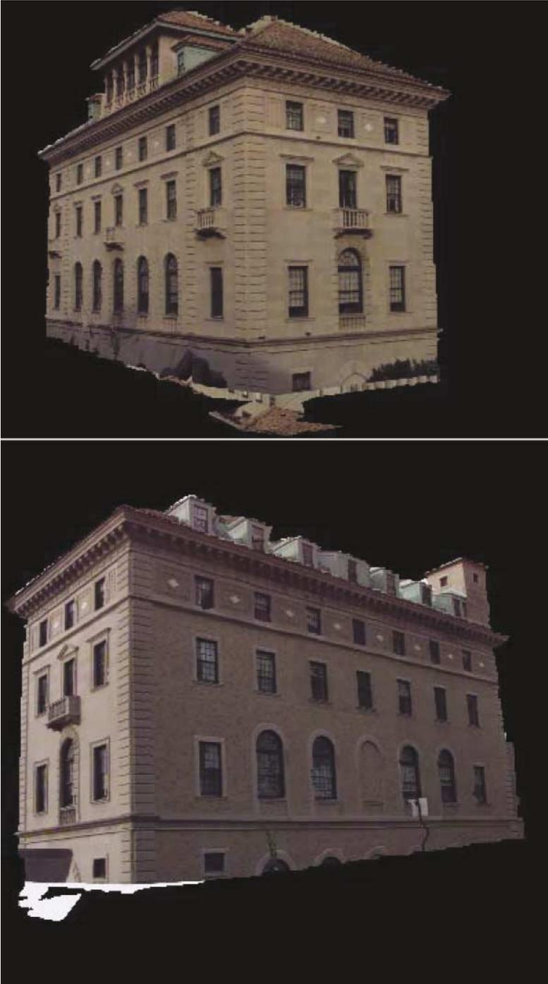
**FIG. 20.** Results. Images texture-mapped on 3-D model assuming final pose (two views of the model). The texture map, visually verifies the accuracy of our method and presents the true geometric model of the scene enhanced with the photometric observations.
