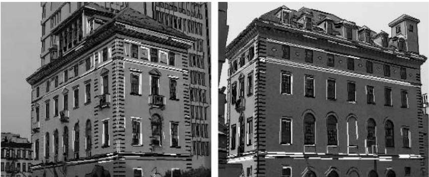
**FIG. 19.** Results. Projected 3-D lines on the images after final pose estimation (shown in green in color or white in black-and-white printing). The extracted 2-D lines are shown in red in color or black in black-and-white printing.
