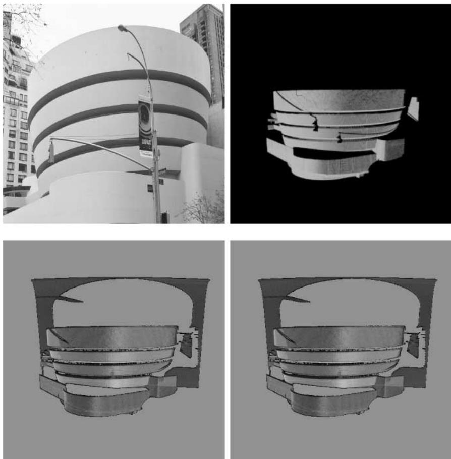
**FIG. 8.** Guggenheim Museum. Top row: Two-dimensional photograph and dense range scan (first view). Bottom row: Segmented range scans (first and second view). Each segmented surface is displayed with a different color. The points which failed the initial *Point Classification* step are displayed in red.
