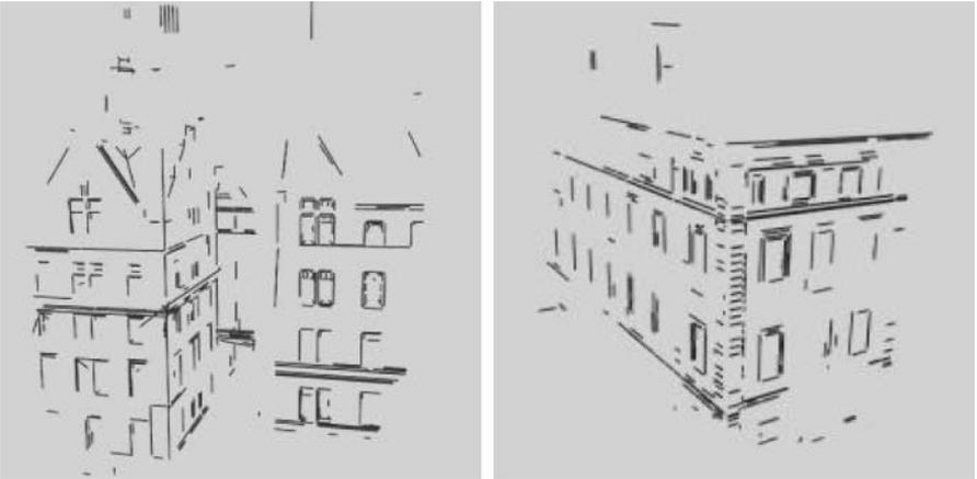
**FIG. 10.** 3-D lines produced by intersection of neighboring 3-D planes. Major features (such as wall and window borders) have been captured. Teachers College (left) and first view of Casa Italiana (right).
