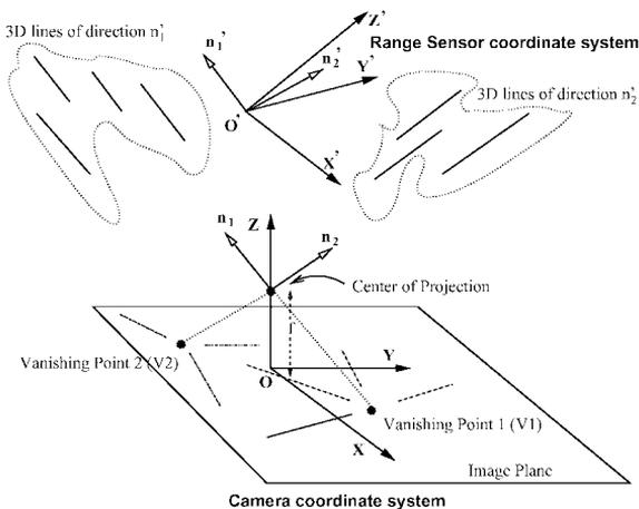
**FIG. 15.** Two vanishing points. The 2-D lines which correspond to parallel 3-D lines of direction  $\mathbf{n}_i$  intersect at a common vanishing point  $V_i$  on the image plane.
