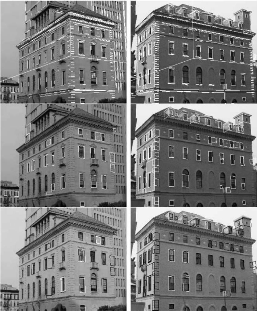
**FIG. 18.** Results. (Top row) 2-D images and clusters of 2-D lines, where different colors correspond to different vanishing points (two views of the building shown). (Middle row) Extracted 2-D quadrangles. (Bottom row) Extracted 2-D quadrangles (shown in red in color or black in black-and-white printing) and  $Q_{match}$ , matched 3-D rectangles projected on images after coarse pose estimation (shown in green in color or white in black-and-white printing).
