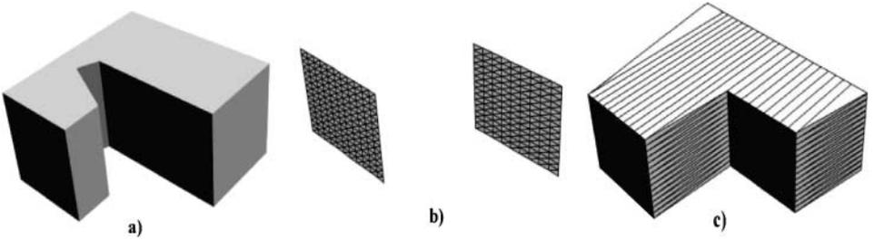
**FIG. 11.** Solid modeling concept. (a) Solid block being sensed, (b) Mesh generated by the measured 3-D points. (c) Partial solid model construction formed by sweeping mesh surfaces along the sensing direction.
