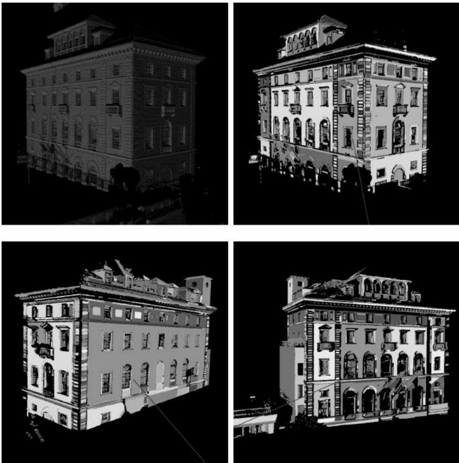
**FIG. 6.** Casa Italiana. Top row: Range and segmented images (first view). Bottom row: Segmented images (second and third view). Each segmented surface is displayed with different color. The points which failed the initial *Point Classification* step are displayed in red (the large segmented wall on the second view is not red). Color versions of all images of this paper can be found at <http://www.cs.columbia.edu/robotics/CVIU>.
