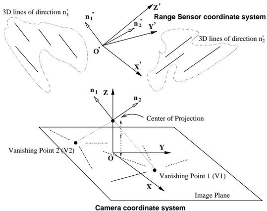
Figure 4: Two vanishing points. The 2-D lines which correspond to parallel 3-D lines of direction  $\mathbf{n}_i$  intersect at a common vanishing point  $V_i$  on the image plane.
