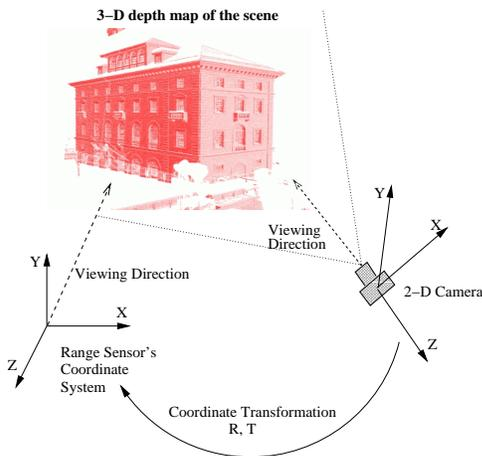
Figure 2: The pose estimation problem. The 3-D model of the scene is represented in the coordinate system of the range sensor. The image taken from the 2-D camera needs to be registered with the 3-D model.
