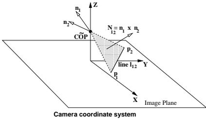
Figure 1: Representing 2-D points and lines as antipodal-points on the Gaussian sphere. A point is represented by the pair of unit vectors  $\pm \mathbf{n}_i$  and a line by the pair  $\pm \mathbf{n}_1 \times \mathbf{n}_2$ .
