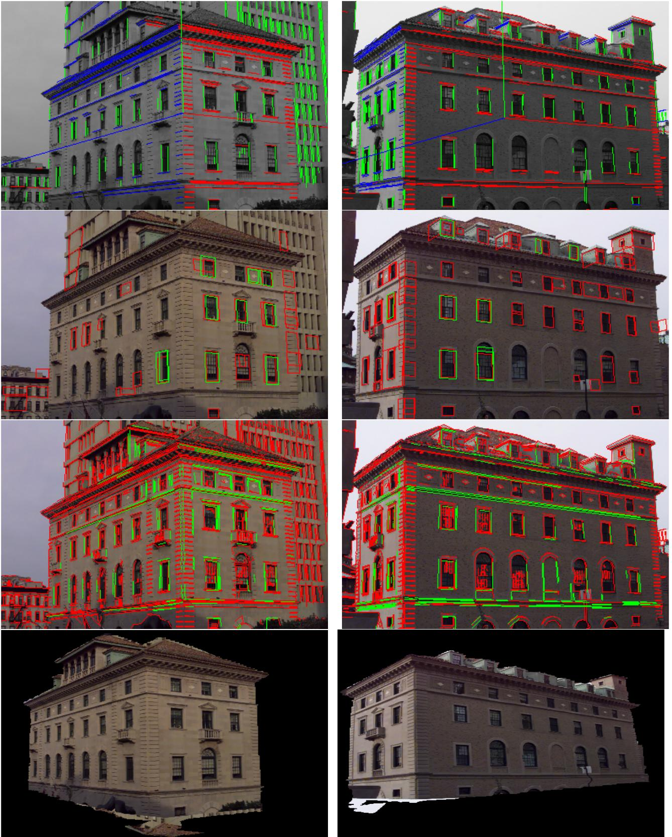
Figure 6: **Results.** a,b) 2-D images and clusters of 2-D lines, where different colors correspond to different vanishing points. c,d) Extracted 2-D quadrangles (shown in red) and  $Q_{match}$  matched 3-D rectangles projected on images after coarse pose estimation (shown in green). e,f) Projected 3-D lines on the images after final pose estimation (shown in green). The extracted 2-D lines are shown in red. g,h) Images texture-mapped on 3-D model assuming final pose.
