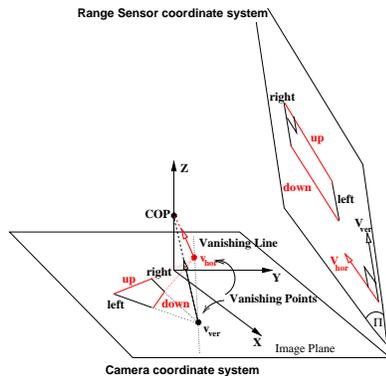
Figure 3: 3-D rectangle formed by lines parallel to the scene directions  $V_{ver}$  and  $V_{hor}$  and its corresponding 2-D quadrangle formed by 2-D lines which meet at the image vanishing points  $v_{ver}$  and  $v_{hor}$ .
