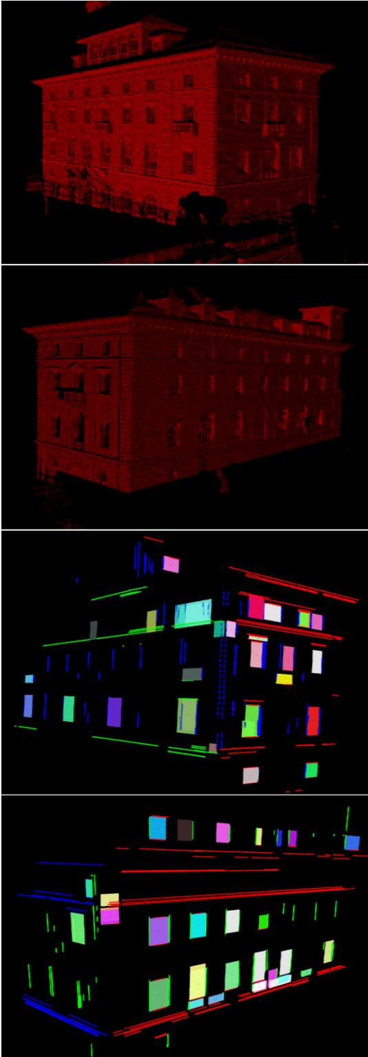
Figure 5: a,b) Range scans of scene. c,d) Clusters of 3-D lines (color encodes different directions) and extracted 3-D rectangles (rectangles are rendered as solids of different color for clarity).
