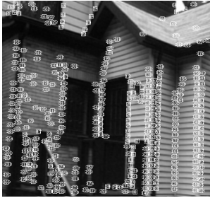
Figure 4.10: The features selected in the first frame of the real house stream (figure 4.9)
