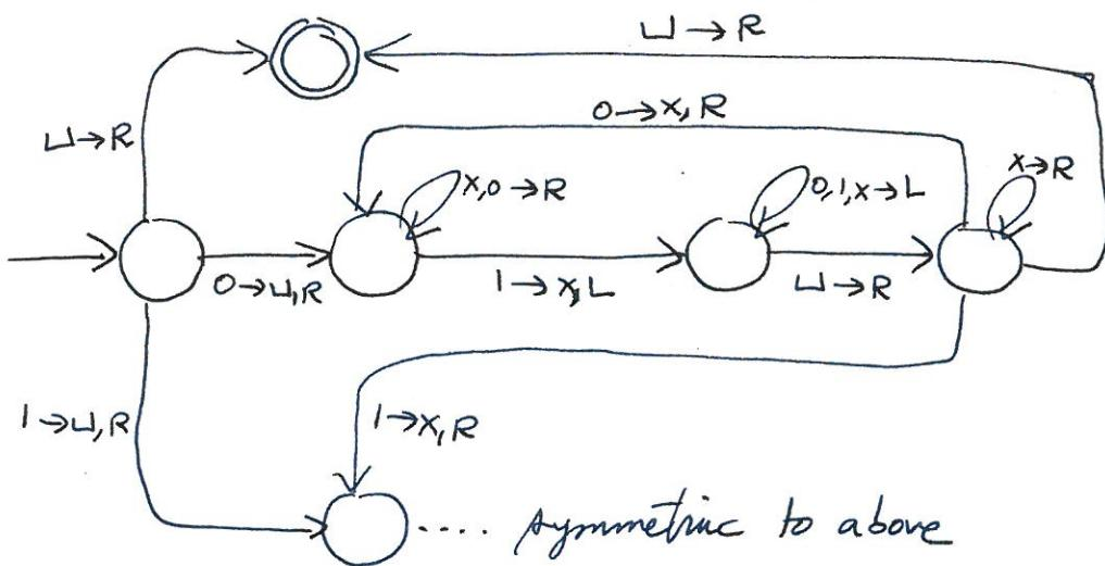
Find the first unmarked bit. If it's 0, mark it and look for a 1. Mark the 1, and go back all the way to the left. Repeat. Transitions not shown go to reject.
