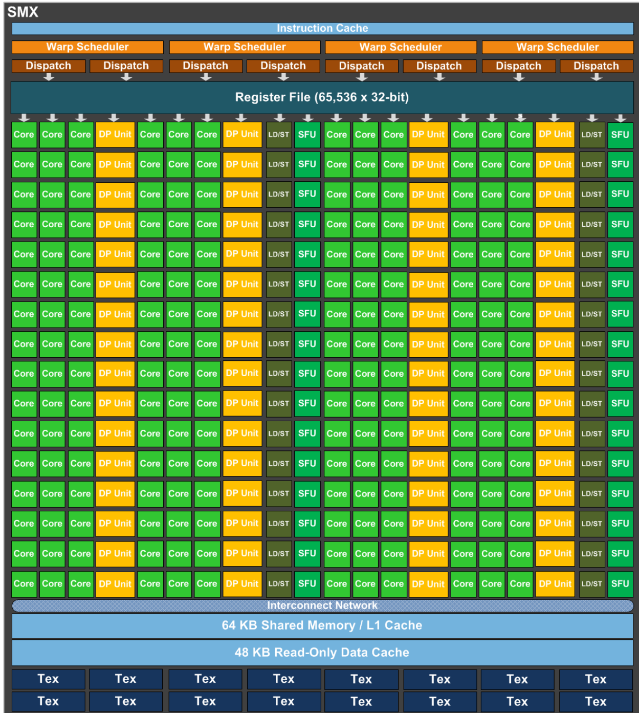
SMX: 192 single-precision CUDA cores, 64 double-precision units, 32 special function units (SFU), and 32 load/store units (LD/ST).
