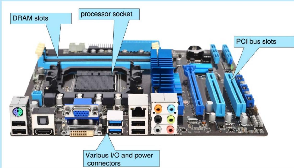
This board is a fully-functioning computer, once its slots are populated. It consists of a processor socket containing a CPU, DRAM sockets, PCIe bus slots, and I/O connectors of various types. Even the lowest-cost general-purpose CPU contains multiple cores. Some motherboards contain multiple processor sockets. More advanced computers allow more than one system board, creating NUMA systems.
