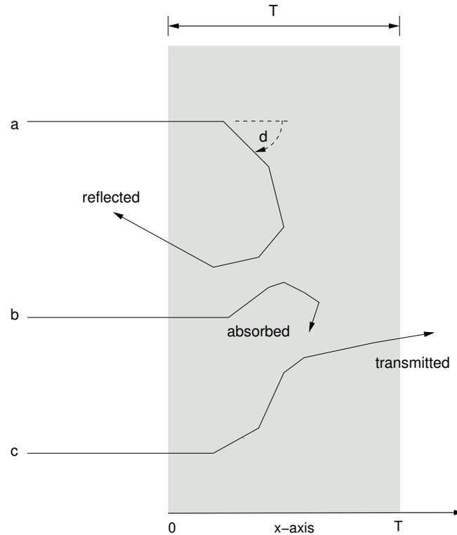
Figure 8.9: Particle interaction with metal plate of thickness  $T$ . Particles have an initial direction perpendicular to the plate and upon reaching it, they interact with its atoms. The result of this interaction is that a particle may eventually be reflected, absorbed, or transmitted through the plate.
