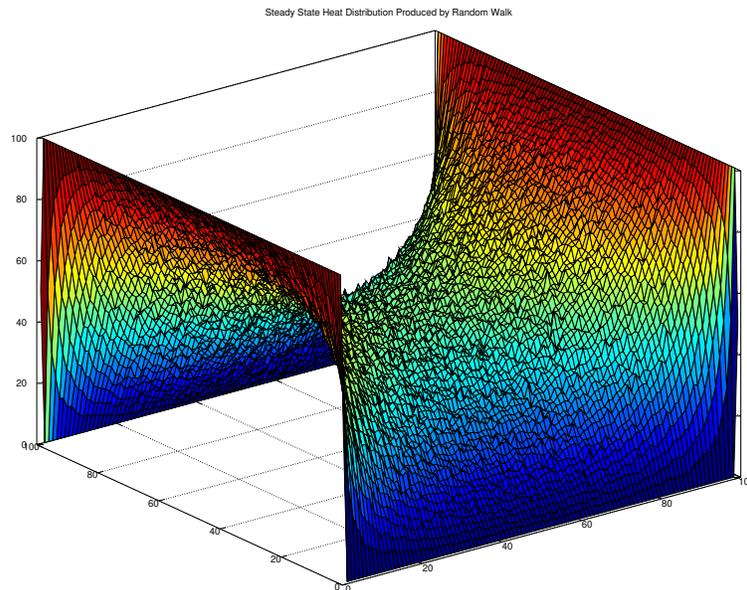
Figure 8.12: Visualization of the result of a random walk solution to the heat diffusion problem in a 2D plate in which the temperature is fixed at 100° C along the east and west edges and 0° C along north and south edges.
