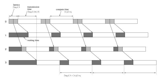
Figure 6.5: Overlap of computation and communication in the first four iterations of the parallel version of Floyd's algorithm, with process 0 responsible for the first 4 rows of the matrix. The figure shows how the transfer of a message overlaps the computation of the sending process.
