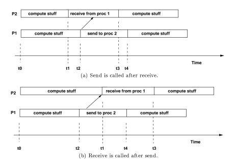
Figure 6.4: Two processes in a point-to-point communication. In Figure (a), the process calls *receive* before the sending process has sent anything. In (b), the sending process calls *send* before the other process has called *receive*.
