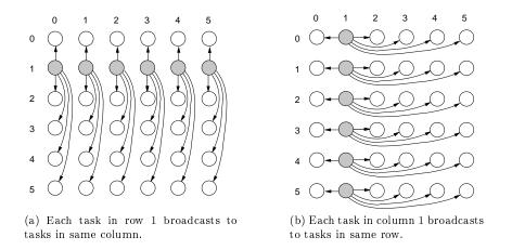
Figure 6.2: Row and column broadcast communication pattern in parallelization of Floyd's algorithm
